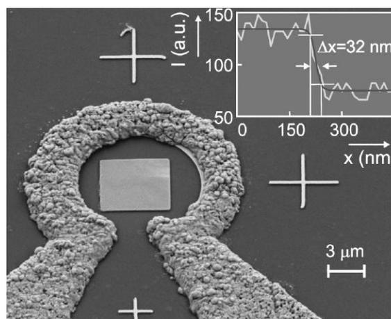
Fig. 2 Microcoil for observation of ultrafast magnetic switching in synchrotron based PEEM.
