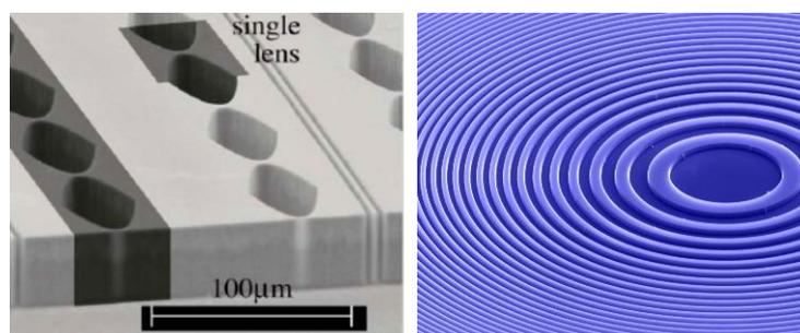
Fig. 3 Refractive (left) and diffractive (right) high resolution x-ray lenses used at microscopy and nanoprobe beam lines.
