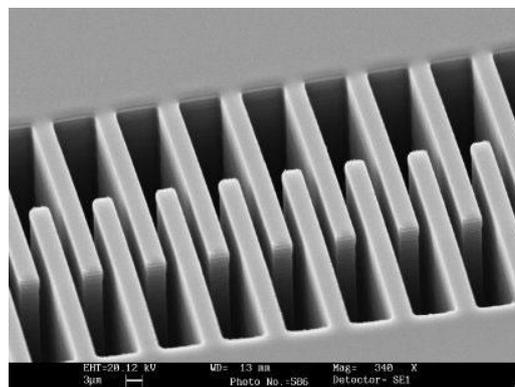
Fig. 16 MEMS comb drive produced by DRIE
