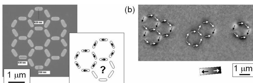
Fig. 1 Geometrically frustrated magnetic kagome ice structures created by electron beam lithography. (a) SEM images and (b) synchrotron PEEM images of kagome ice structures with three, two and one ring revealing the magnetization state.
