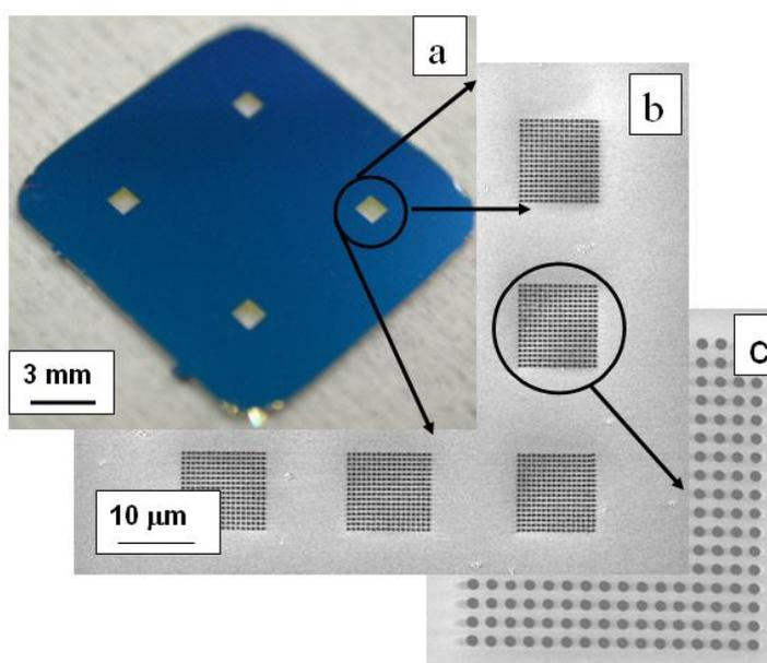
**Fig. 12** Nanopore membrane chip device (a) for research on individual membrane molecular complexes with (b) structured membrane area with nanopore arrays with (c) diameter/pitch 330/600 nm, fabricated by NIL in combination with photolithography and micromachining.
