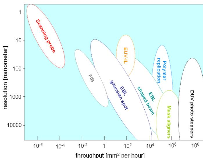
Fig. 4 Schematic comparison of nanolithography methods with respect to resolution and speed/throughput. Techniques for pattern origination show a clear dependence of throughput and resolution (diagonal shape), while the speed of replication techniques is independent on structure size (vertical shape).
