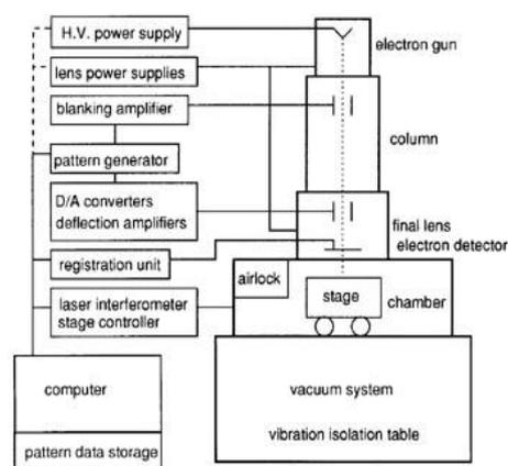
Fig. 5 Schematic layout of an electron beam lithography system (taken from <sup>1</sup>)
