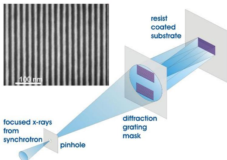
**Fig. 11** Schematic view of extreme UV interference lithography and SEM image of 25 nm period resist structures produced by EUVIL.
