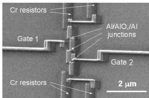
**Fig. 17** SET device made by e-beam lithography and sloped liftoff technique (courtesy T. Weimann, PTB Braunschweig)
