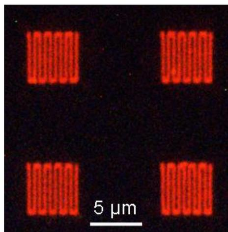
**Fig. 8** Fluorescently labelled phospholipids patterned on a polystyrene surface with a half-pitch of 250 nm (Courtesy Karlsruhe Nano Micro Facility).
