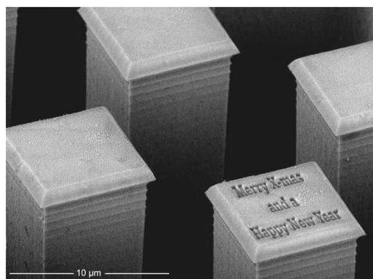
Fig. 6 Nanostructures (text) written onto microstructures illustrating the high flexibility of FIB lithography (courtesy T. Rohbeck, FH Bremen))
