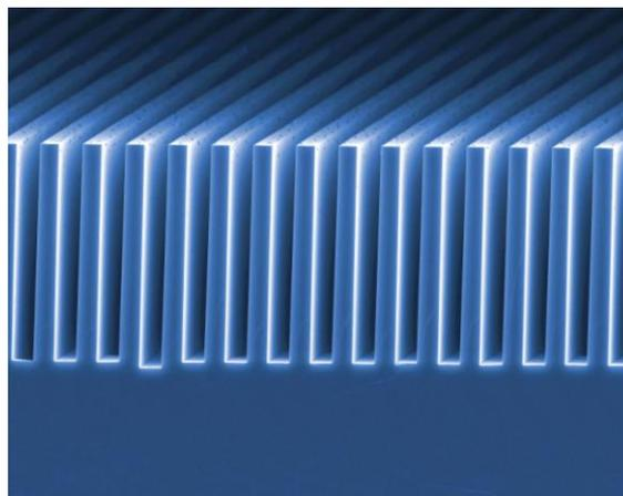
**Fig. 14** Examples of high aspect ratio silicon microstructures produced by anisotropic wet etching. The structure period is 4  $\mu\text{m}$ .
