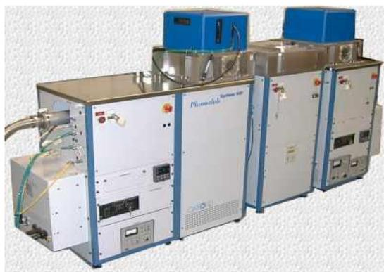
Fig. 15 Combined RIE and PECVD cluster tool (courtesy Oxford Instruments Inc.)
