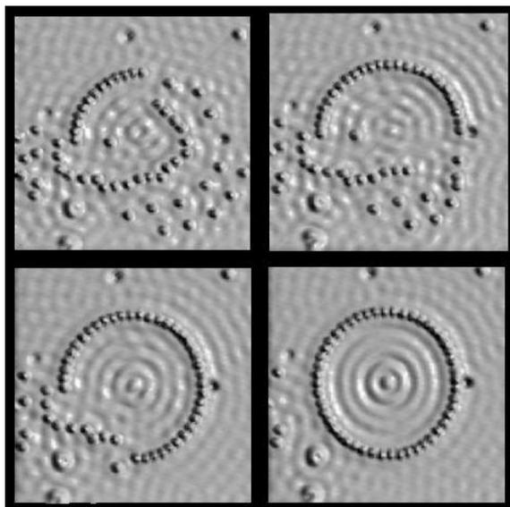
**Fig. 7** 48 iron atoms arranged by STM on the surface of a copper substrate. These images show the various stages of the process (M.F. Crommie, C.P. Lutz, D.M. Eigler, *Science* **262** (1993) 218-220)
