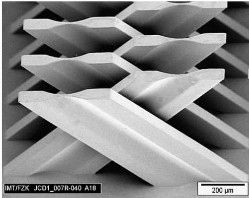
**Fig. 10** Refractive lens for hard x-rays fabricated by the LIGA process using two tilted exposure steps (J. Mohr, V. Nazmov, Forschungszentrum Karlsruhe).
